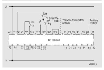
Two-channel emergency stop circuit without cross fault detection. Activation via On pushbutton. - - - Jumper X5 - X6:
