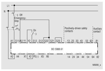
Two-pole emergency stop circuit with emergency stop control device in the supply circuit.
