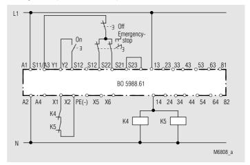
Contact reinformcement by external contactors with reduced safety
