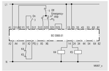
Contact reinforcement by external contactors, two-channel.
