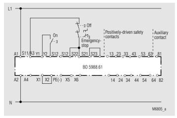
One-channel emergency stop circuit. This circuit does not have any redundancy in the emergency stop control device circuit.
