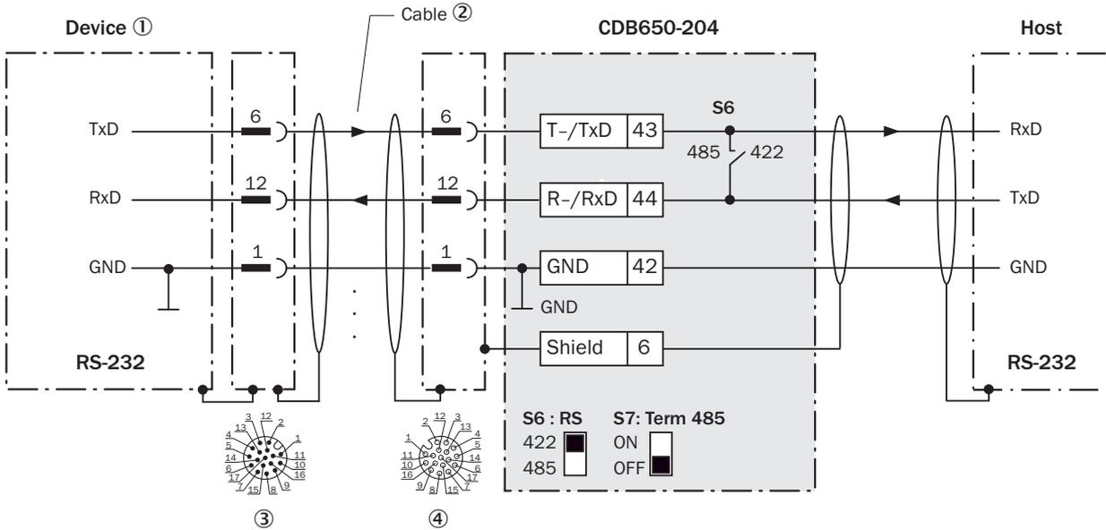
Figure 15: Wiring the RS-232 data interface
