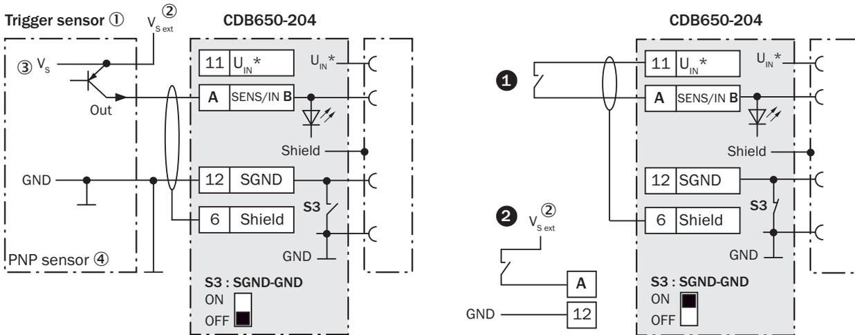
Figure 19: Left: trigger sensor connected volt-free and powered externally. Right: alternative switch, ❶ powered by CDB650-204 or ❷ connected volt-free and powered externally. Switch setting S3 as in the left-hand figure.
