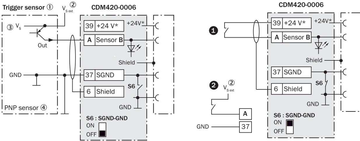
Figure 30: Left: trigger sensor connected volt-free and powered externally. Right: alternative switch, ❶ powered by CDM420-0006 or ❷ connected volt-free and powered externally. Switch setting S6 as in the left-hand figure.
