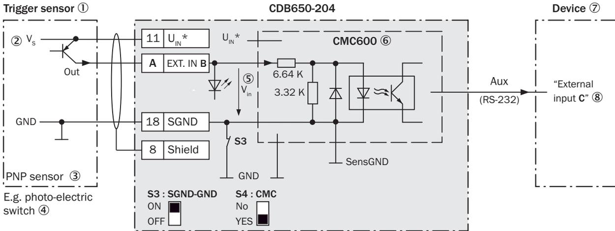
Figure 20: Trigger sensor powered by the CDB650-204
