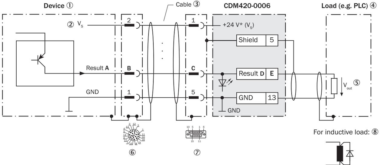
Figure 33: Wiring the switching outputs
