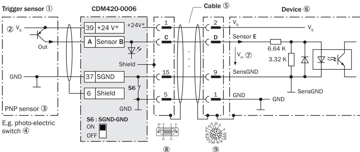
Figure 29: Trigger sensor powered by the CDM420-0006
