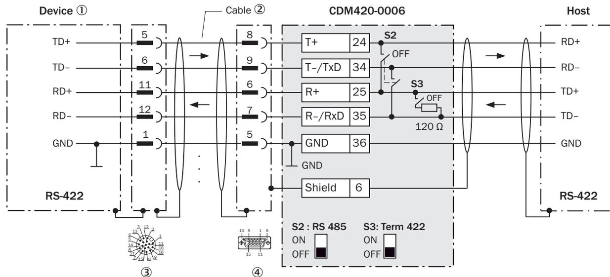
Figure 27: Wiring the RS-422 data interface
