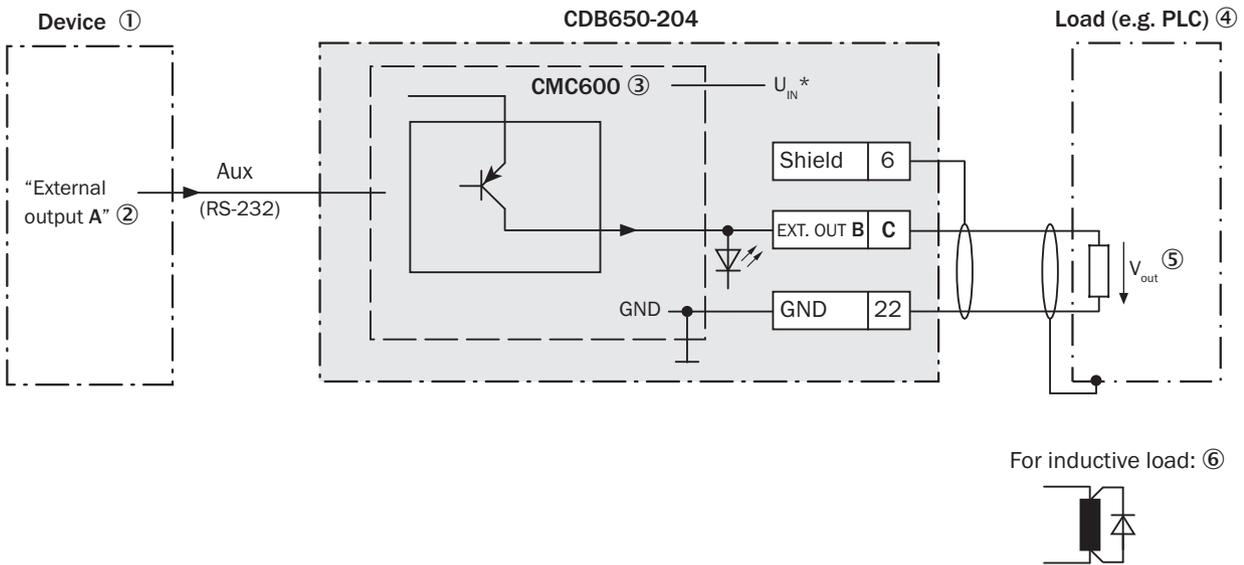
Figure 23: Wiring external switching outputs
