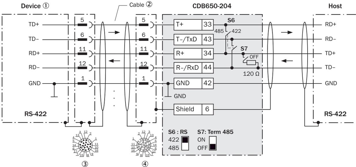
Figure 16: Wiring the RS-422 data interface
