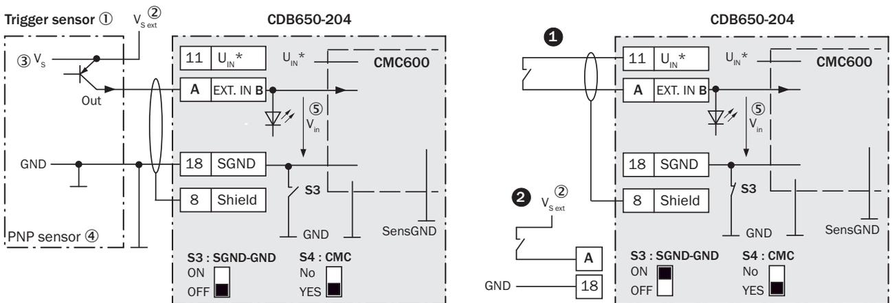
Figure 21: Left: trigger sensor connected volt-free and powered externally. Right: alternative switch, ① powered by CDB650-204 or ② connected volt-free and powered externally. Switch setting S3 as in the left-hand figure.
