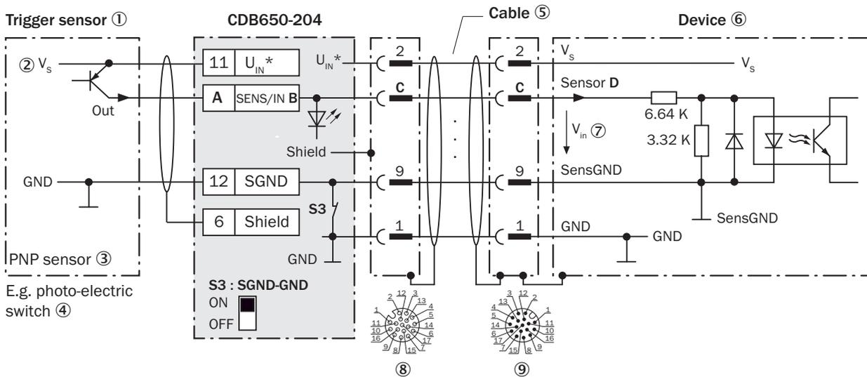
Figure 18: Trigger sensor powered by the CDB650-204
