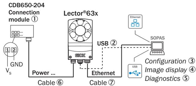
Figure 10: General connection principle
