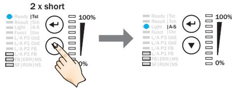
The bar graph shows the progress of the Auto-Setup function in percent. 100% means the Auto-Setup has finished. The color of the “Auto-Setup” LED now signals the success status.
