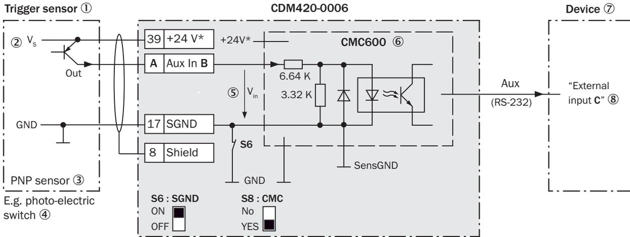
Figure 31: Trigger sensor powered by the CDM420-0006
