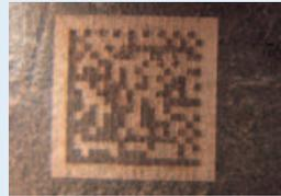
To achieve an optimum contrast between code and background, the laser not only creates the actual code but also modifies its background. This minimizes interference structures, such as those that occur in cast materials or polished, shiny surfaces. This is known as cleaning.
