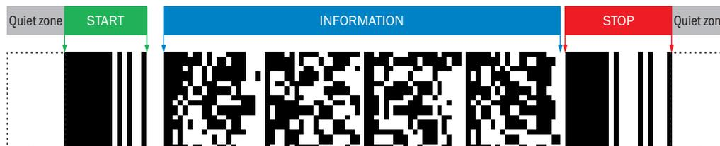
Basic components of a stacked code with quiet zones: start and stop characters and the encoded information
