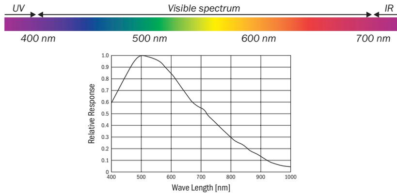
Example of the spectral sensitivity of a camera chip: can be used throughout the entire visible range.
