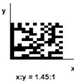
Checks the ratio between length and width of the code. If the code is stretched or compressed in length or width, it is given a poor rating for its axial non-linearity. | A (4.0)<br>B (3.0)<br>C (2.0)<br>D (1.0)<br>F (0.0) | AN ≤ 0.06<br>AN ≤ 0.08<br>AN ≤ 0.10<br>AN ≤ 0.12<br>AN > 0.12                                          | •             | •       |           | •                                                                                |
