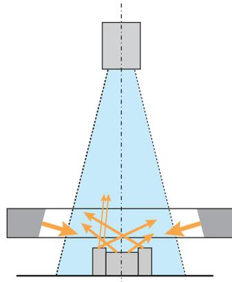
The light source is aligned in relation to the camera in such a way that the majority of the reflected light is not parallel to the optical axis of the camera. Only light that reflects on the edges runs parallel and thereby falls on the image sensor of the camera. As a result, the edges of the object are illuminated while the background remains dark. The dark field illumination method is particularly well suited to dot peening.
