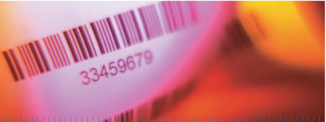
Almost all code types can be extended to include check digits, which are used to verify the plausibility of the read result. The check digit is calculated from the read result of the barcode according to a defined formula and compared with the check digit value that was included in the barcode. If both values match, the content of the code is output. If they do not match, the reader outputs the result “no read”. This avoids any misinterpretation and, consequently, any misinformation.
