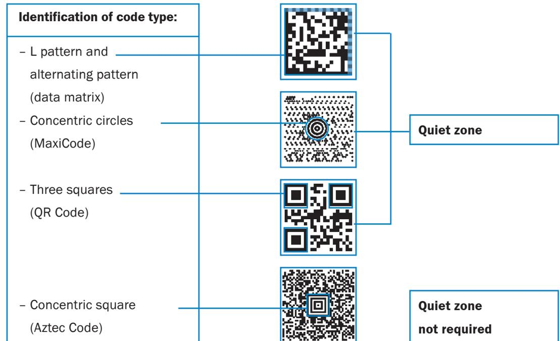
Matrix codes consist of a data field and additional, code-dependent finder patterns. These finder patterns allow the code on an object to be located and identified.
